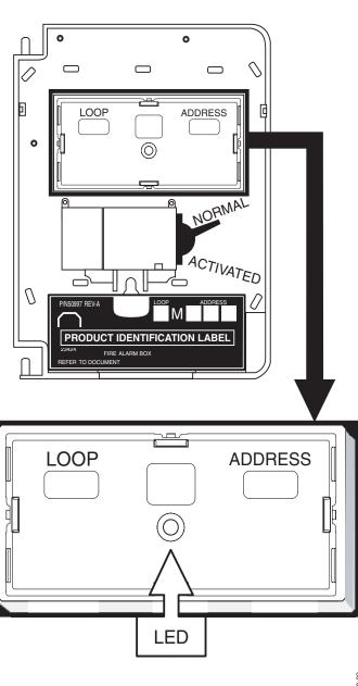
Note – Opening the pull station door will <u>not</u> activate or deactivate the alarm switch.
